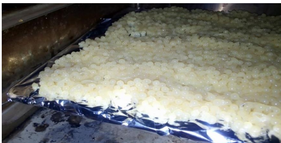
Plate 2: Washed and drained beads spread on a dryer tray ready for drying in an oven
